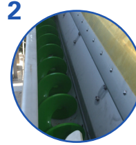
2 Compacting screw Obtaining a compact waste and reducing volumes by more than 50%
