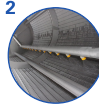
2 Washing ramp Optimum cleaning of drum
