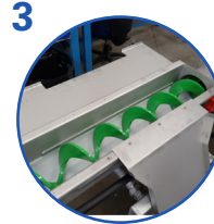
3 Compactor (RC version) Optimized conditioning of trash
